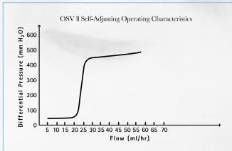
By adjusting the size of the valve passageway, the OSV II system works to maintain a flow rate of approximately 20 ml/hr (consistent with the natural rate of production in adults).
